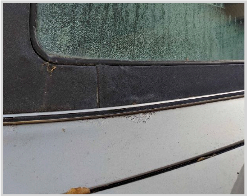
Also on the Silver Wraith II, typical damage can be found beneath the rear glass and above the bodywork.
