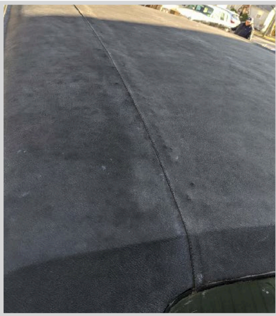
This Silver Wraith II. exhibits many of the faults found on original Everflex cars, from corrosion to splitting to bunching up and even some lumpiness!
