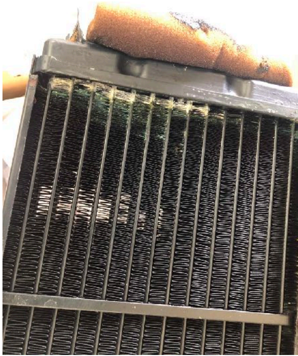
Heater Core with Corrosion Visible
