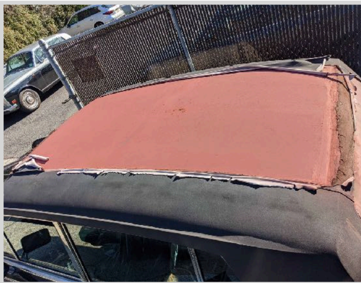
Original vinyl peeled away and without any adhesive, this head is still in restorable condition.
