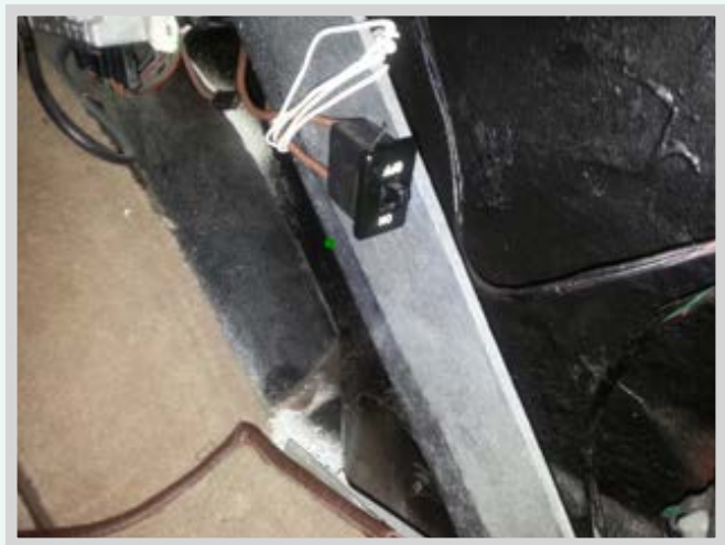
Engine Run Sensor Override Switch Connected to the Fuel Pump Relay Socket
