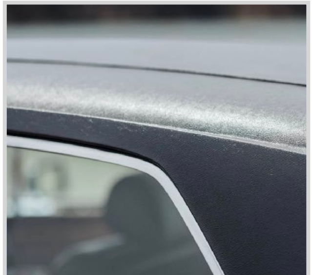
Note how the Everflex (if well applied) perfectly encapsulates the accents and shapes in the metalwork on the Corniche FHC models.
