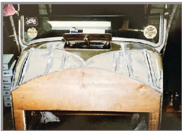
The Body Being Fitted to Ghost's Firewall.
