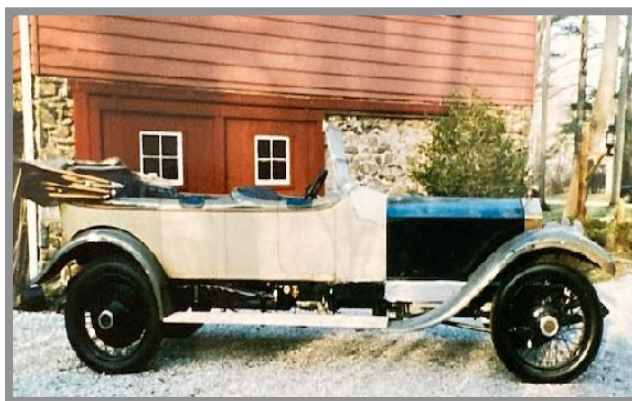
The Simplex Body Placed on the Ghost’s Chassis.
